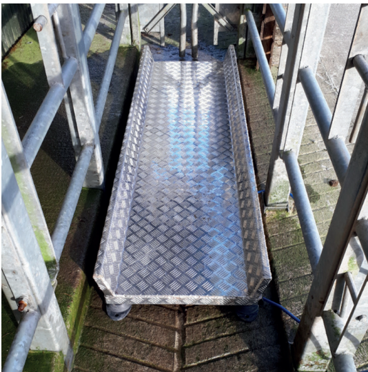
Figure 2. Weighing platform placed correctly at the top of a cattle crush.
