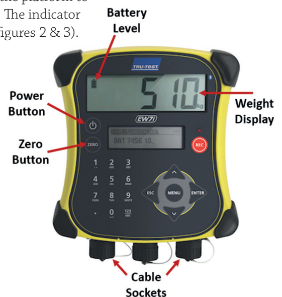
Figure 4. Tru-Test Eziweigh 7 indicator functionality.
