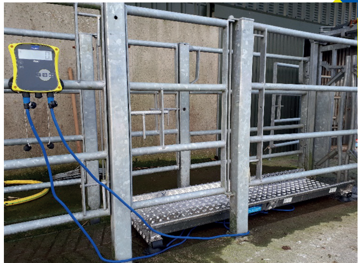
Figure 3. Indicator in a safe position and excess cable from load bars underneath platform.
